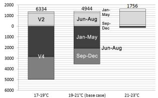
Figure 6: No. of hours when the OT is >26°C in V2 (kitchen and dining-room) (light grey) and no. of hours when the OT is <19°C in V4 (bedrooms) (dark grey); summing up to the no. of hours when the OT is <19°C or >26°C; according to different temperature set points
