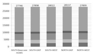
Figure 3: AHED (kWh) per volume (V5(basement) at the top and V1(living-room) at the bottom); summing up to AHED (kWh); according to different orientations
